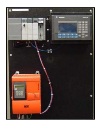
This is the Sew Eurodrive DeviceNet / Profibus control system. It is composed of a Sew Eurodrive AC inverter drive that accepts all its commands through an Allen Bradley DeviceNet or Siemens Profibus interface. All of the systems functions are controlled via the AB Panelview 550 touch screen. Through the touch screen, you can select either the AB DeviceNet or the Siemens Profibus interface for system communications control as well as all drive functions.
